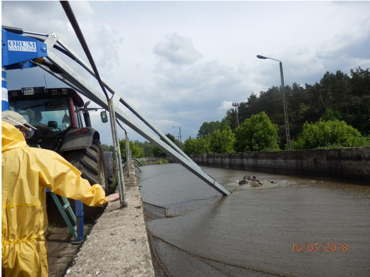
Fig. 4. Slurry mixing and acidification using ORUM system [Source: ITP, author: J. Barwicki]
