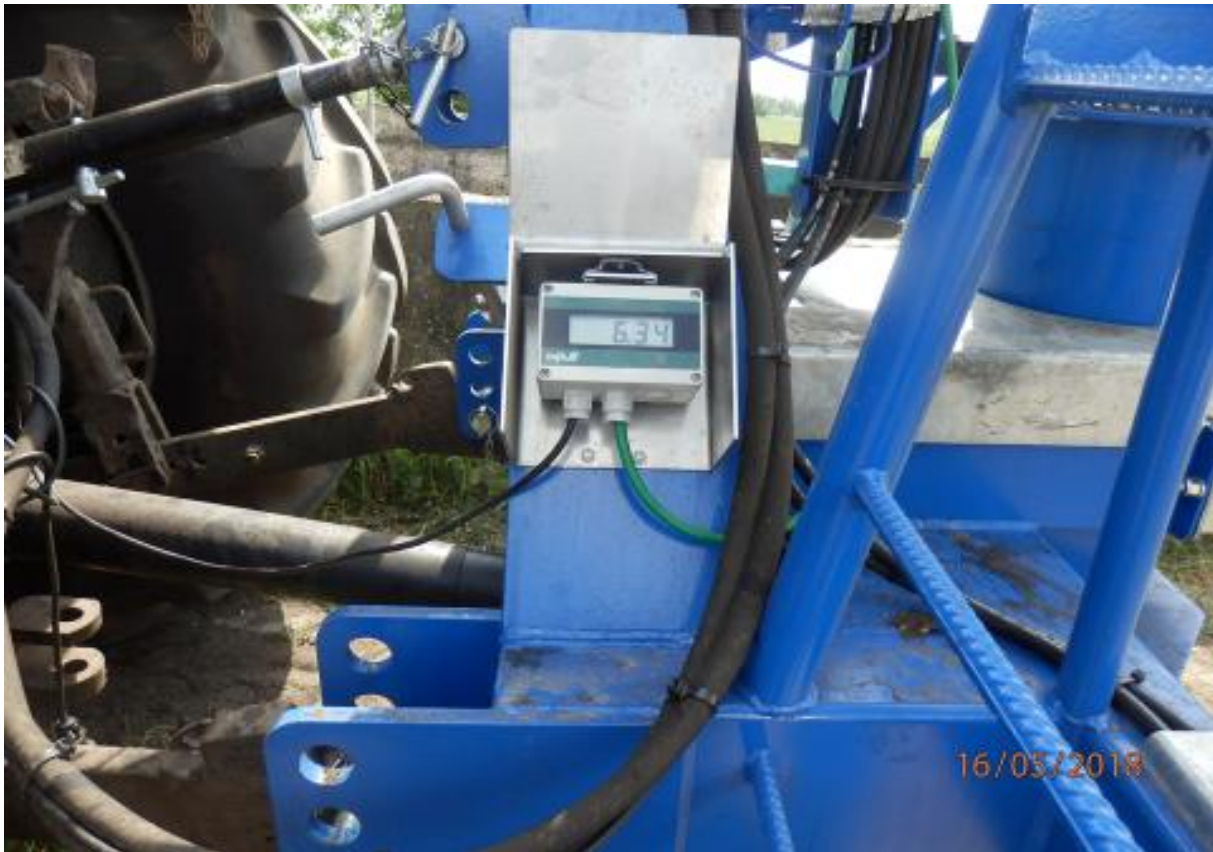
Fig. 5. In line reading of pH value of slurry during acidification of slurry in ITP Biebrza farm [Source: ITP, author: J. Barwicki]
